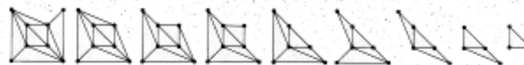
Serious pruning shows that V + F - E of the original solid equals that of a single triangle.
